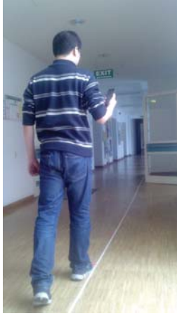
Fig. 1. To discover the step length model, a large number of experiments are implemented by volunteer. The step length and frequency are calibrated by measuring tape and metronome. The acceleration data are collected by smartphone.
